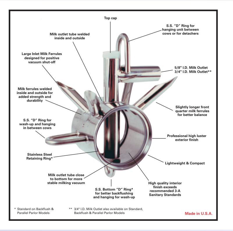
Many of the stainless steel claws available on the market today are welded only on the inside of the claw. The milk ferrules and milk outlet tube of the IBA Top Unloading Claw are welded on both the inside and outside to increase the strength and durability. Except for replacing an occasional side window or gasket, this claw is virtually maintenance free.
